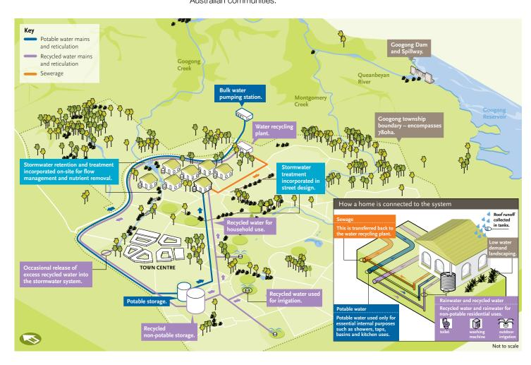
The design concept has a number of underlying principles, strongest of which is the protection of the Googong Dam, and it should be noted that the IWC is separate from, and does not discharge to, the Googong Dam.
